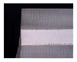
All fabrics having thread diameters < 250 μm and mesh openings < 500 μm can be ultrasonically welded
