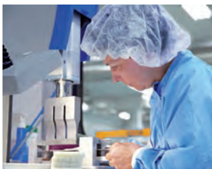
Class 7 cleanroom according to ISO 14644
