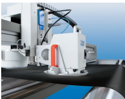
In-line testing of air permeability
